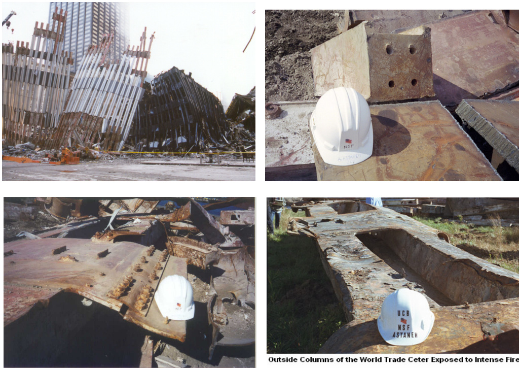
Figure 6. Views of the damaged components of the World Trade center towers 1
